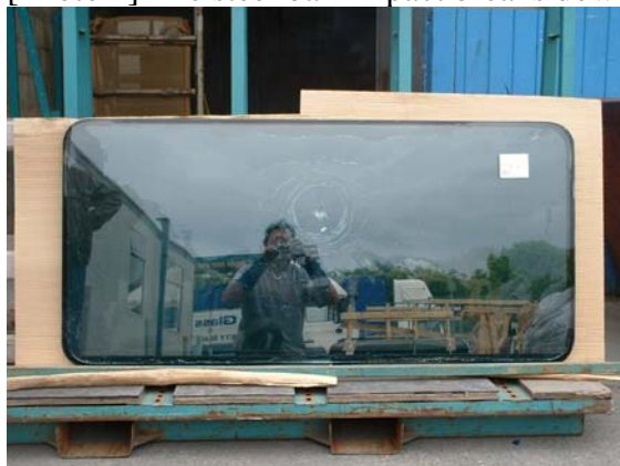
... while the internal panel remains intact, protecting the vehicle occupants [photo 2].
