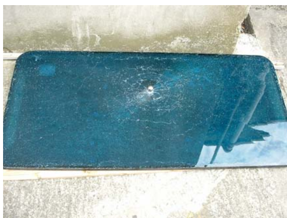
[Photo 1] The steel ball impact breaks down the external panel of the unit....
