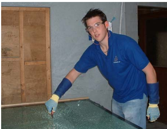
(Picture shows John testing the break pattern in toughened safety glass)
